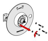
3. Remove flange screws Unscrew the flange screws
